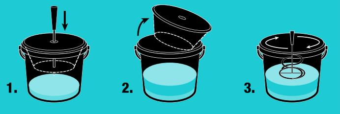
1. Pierce the centre of the lid on the top chamber and push through to pierce the centre of the base also. Allow the material (hardener) to fully drain from the top container into the base. This will normally take between 3 and 5 minutes.
